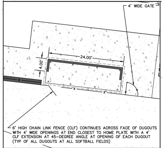
**REVISE** DUGOUT INSET per the revision shown below to align the proposed 45-degree fence opening with the far-left dugout column.
