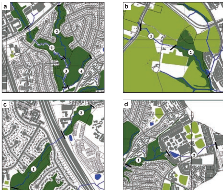
Figure 21: Various physical factors control how survey reaches are delineated. (a) Survey reaches based on the confluence of stream tributaries. (b) A long tributary split into \frac{1}{4} mile survey reaches.
