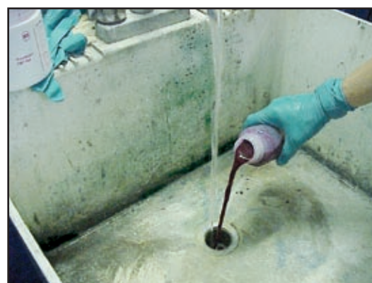
Figure 63: Dye Testing Plumbing (NEIWPCC, 2003)
